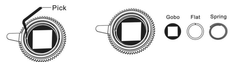
Locate the tab of the spring, and with a precision pick (or similar tool), carefully press the retaining spring inward to relieve the tension. Remove the retaining spring and carefully separate the GOBO from the GOBO Holder. Lastly, remove the flat washer attached to the removed GOBO and attach it to the desired replacement GOBO. Install the replacement Rotating GOBO following the steps above in reverse order.
