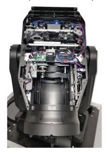
2. Unplug the power and data cable for the module, then remove the four (4) module screws holding the module in place, as indicated by the arrows in the image below. Pull the module gently towards you, taking care to ensure that the module does not catch or snag on any surrounding cables.
