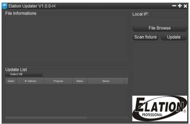
Once opened, it will automatically identify your local IP. Click "Scan fixture" and create a connection. The fixture identity will appear in the Update List on the left side of browser. A connection will fail to establish if the fixture IP and Local IP are not in the same network segment.
