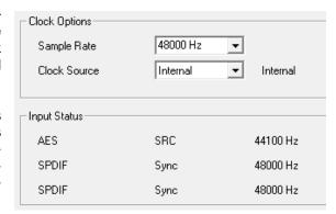
This way, configuring any suitable audio application for digital recording is simple. After selecting the correct input, Digiface AES displays the current sample frequency. This parameter can then be changed in the application's audio attributes (or similar) dialog.
