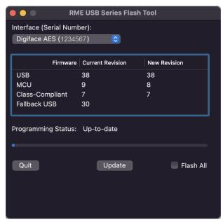
To speed up the process of flashing the app only updates older parts of the firmware. Using the option *Flash All* a complete update can be forced.
