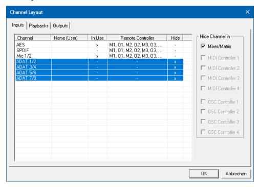
Hidden channels in *MIDI Remote x* are removed from the list of remote controllable channels. Within an 8-channel block of a Mackie compatible control they are skipped. The control therefore is no longer bound to consecutive orders. For example it will control channels 1, 2, and 6 to 11, when channels 3 to 5 are hidden. The same can be done for OSC. With unnecessary channels made invisible for the OSC remote the more important channels are available as one block on the remote.
