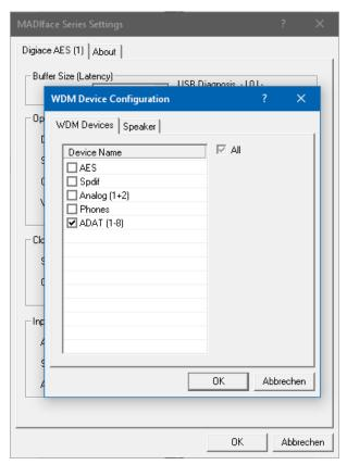
The screenshot to the left shows the multichannel WDM devices available with the Digiface AES after selecting 'Multi-Channel' in the WDM Devices listbox and hitting WDM Configure. In this example the devices ADAT (1-8) is active.
