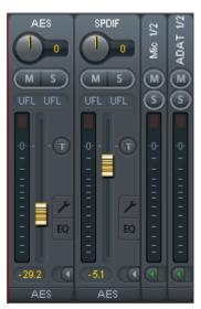
The **arrow symbol** at the bottom minimizes the channel width to that of the level meters. Another click maximizes it again. A mouse click with held Ctrl key causes all channels to the right to enlarge and minimize at once.
