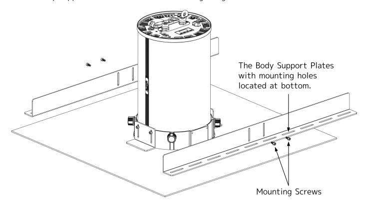
4. Install the entire assembly back into the ceiling at the desired location, making sure that the ends of the Body Support Plates are resting firmly on the Ceiling Support Grid. Secure the Body Support Plates in place using the appropriate hardware.
