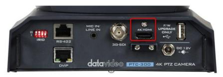
Connect the HDMI OUT to an external connected monitor using an HDMI cable.
