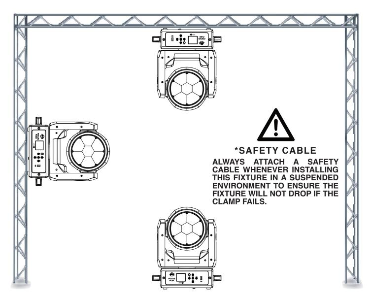
The Focus Flex is fully operational in three different mounting positions, hanging upside-down, mounted sideways on trussing, or set on a flat level surface. Be sure this fixture is kept at least 0.2m (7.9in.) away from any flammable materials (decoration etc.). Always use and install the supplied safety cable as a safety measure to prevent accidental damage and/or injury in the event the clamp fails (see next page). Never use the carrying handles for secondary attachment.
