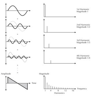
Additive components of the Sawtooth wave
