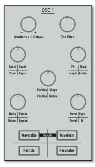
The Oscillator Section for Oscillator 1
