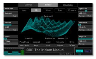
(!) The wavetable position can be dragged vertically in the graphical wavetable representation.
