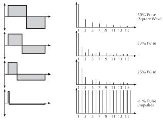
Additive components of Pulse wave with different pulse widths
