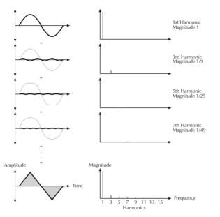
Additive components of the Triangle wave
