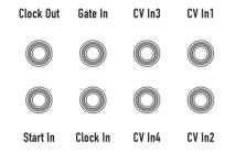
CV/Gate and Clock connections on the Iridium Keyboard rear panel
