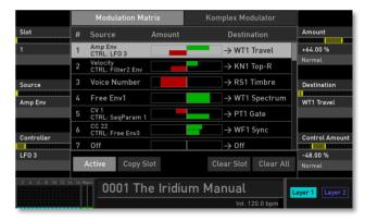
This page shows all modulation assignments in a list. You can set up to 40 assignments.
