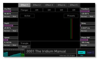
• For the typical Flanger effect sound the **Dry/Wet** parameter should be set to 50%.
