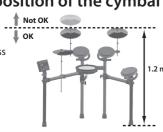
Attach the cymbal rods so that they face straight up, to prevent the drum stand from falling
