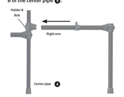
**2–4.** Once the pipe is fully inserted, tighten the bolts (2) of holder B with the drum key.
