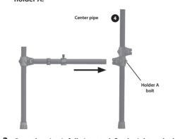
**2–2.** Once the pipe is fully inserted, firmly tighten the bolts (2) of holder A with the drum key.
