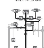
\* Use cable clips 10 to fasten the cables so that they don't obstruct your playing. We recommend attaching the clips in the locations shown with
