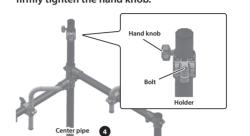
**5–3.** Insert the top pipe into the holder, and use the drum key
