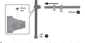
1–2. Once the pipe is fully inserted, firmly tighten the bolt
