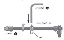
4-3. Use the drum key to loosen the bolt of the L-shaped pipe holder for the right arm (5), and insert the L-shaped pipe 10.
