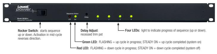
The low voltage rackmount sequencer is used in conjunction with remote power controls (RPCs) to provide time-delayed activation and deactivation of connected equipment, often located in another rack, room or building. The sequencer can also control accessory systems such as projector screens, lighting or blinds. To initiate sequencing, use the rocker switch on the front panel or connect an external switch to the rear terminal block for remote activation.
