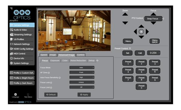
The Advance Image > Focus tab allows you to adjust the various focus settings, including Auto Focus, AF Zone, Auto Focus Sensitivity, Focus Lock, & Focus Limit.
