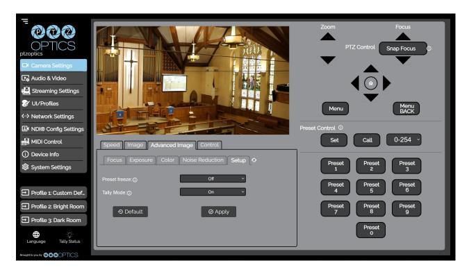
The Advanced Image > Setup tab allows you to change the Image Style and Toggle Tally Mode on / off.
