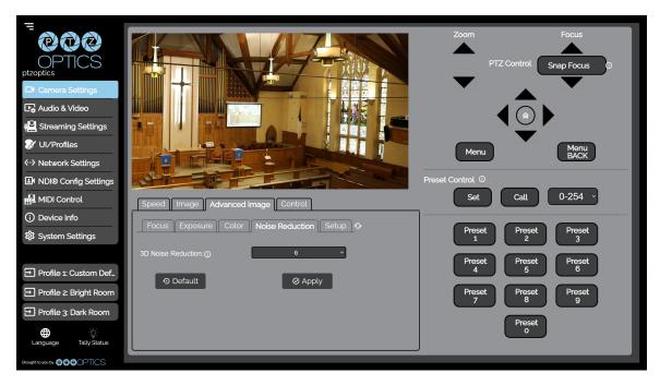
The Advanced Image > Noise Reduction tab allows you to fine tune the 2D & 3D Noise Reduction setting.
