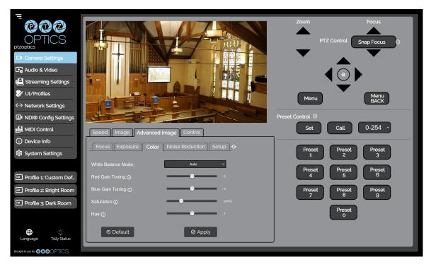
• The **Advanced Image > Color tab** allows you to fine tune the camera's white balance and color tint settings to adjust for lighting as well as ensuring images from multiple cameras match.
