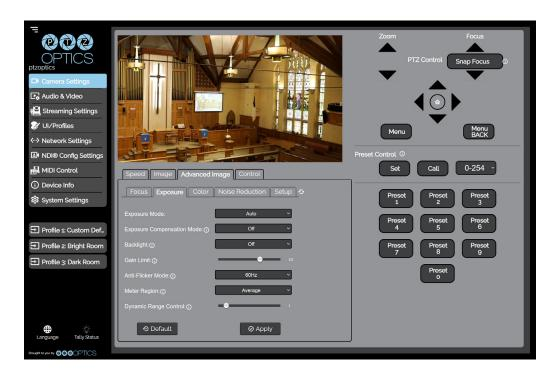
• The **Advanced Image > Exposure** tab allows you to fine tune the camera's exposure settings to ensure image clarity as well as ensuring the images from multiple cameras match.
