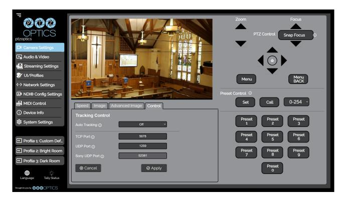
The Control tab allows you to access the camera's TCP, UDP, & Sony UDP control ports.
