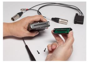
3. Position the A-XLR accordingly, and replace screws.
