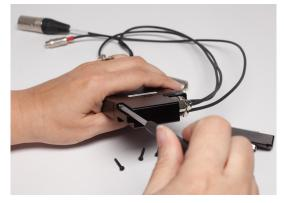
Scomplete the above procedure in reverse to convert from A10-RX-XLR to A10-RX-SL.
