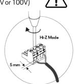
Output mode options (Low-Z or Hi-Z) are configured via the amplifier network interface in the Output>Speaker Preset>Output Mode menu.
