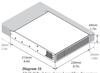
FX Half-Rack **two** channel amplifier dimensions. Shaded area defines ventilation space
