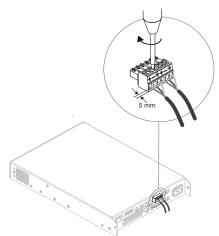
Diagram 8.2: Balanced Input connections
