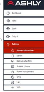
Note: The "Find Me" locator button in the Device menu will continually flash the amplifier's front panel LEDs in a unique pattern until the button is pressed again.
