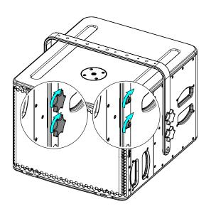
Place on CLADAPT, use the 2 guides. Tight with the fasteners provided with CLADAPT
