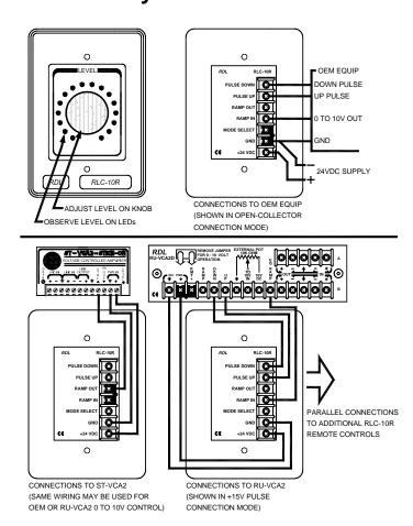
NOTE: Wiring between VCA and RLC-10R must be electrically shielded, either by installation in a metal conduit or using shielded cable. When shielded cable is used without conduit (or in nonmetallic conduit), the shield should be connected to the RLC-10R mounting enclosure.
