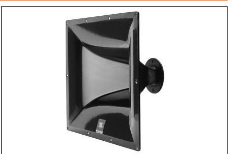
JBL models 2352, 2353, and 2354 are medium format elements of JBL's preeminent family of Bi-Radial<sup>®</sup> horns, providing uniform coverage control over the bandwidth of 630 Hz to beyond 18 kHz, allowing precise control of critical vocal range energy. These medium format horns provide extremely low distortion at typical peak sound pressure levels of 139 dB-SPL at 1m.
