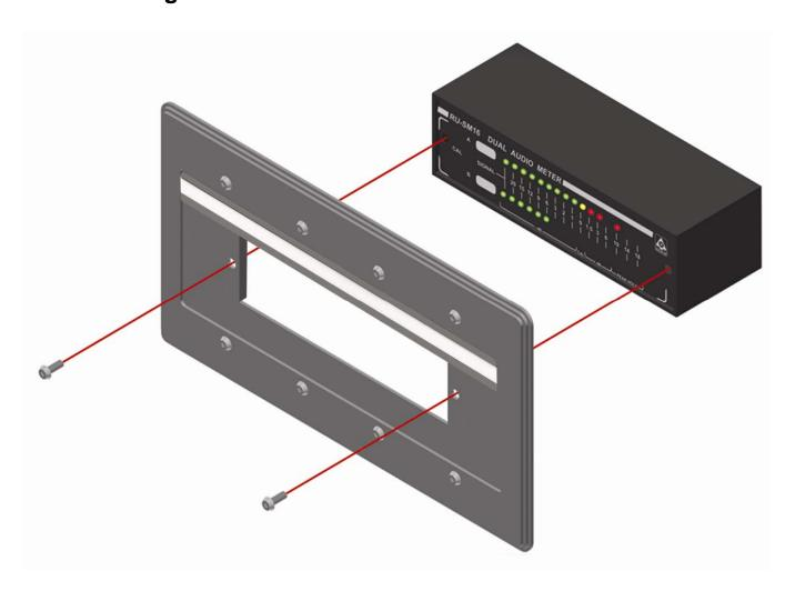
STEP 1: Mount RACK-UP module to the RU-WMP1 panel.
