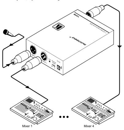
Figure 2: Connecting the 104B 1:4 Microphone DA
