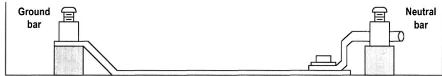
If this loadcenter is to a SUB PANEL, fed from another main panel, the neutral to ground bonding jumper should be disconnected from the neutral bar. The green bonding screw MUST be tightened to maintain ground bar to box bonding. A separate ground conductor MUST be provided back to the main panel.
