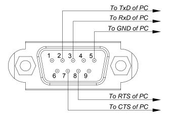
**NOTE 1**: Pins 2, 3, 5, and 6 are used inside the projector.
