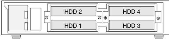
The HDDs should be installed in the proper positions in order as shown above. Do not skip or reverse the order of the HDD positions.
