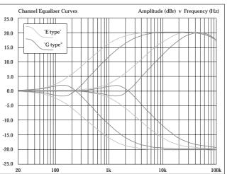
The two parametric bands have selectable characteristics which affect the relationship between frequency bandwidth and gain:
