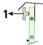
**2- Slide the articulated joint out of the receiver tube by lifting its retaining screw upward.**
