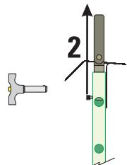
**3- Lock in place using the ball lock pin.**
