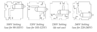
Note. Where the mains voltage is a nominal 230V, the '240V Setting' should be used – not the '230V Setting'!
