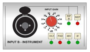
The stepped INPUT GAIN control has a gain range of +6dB to +72dB in 6dB steps.
