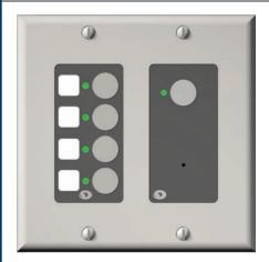
ARC-Mic is a dual-gang controller with an onboard electret condenser microphone and pushto-talk button mounted alongside an SW4 button set. It is typically used as an in-wall paging station, but can be used in other applications such as talkback, intercom, or as a microphone for ambient noise sensing. A dual-gang white mounting plate is included.
