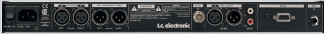
Power Input 100 - 240V Balanced Analog Inputs XLR Balanced Analog Outputs XLR BNC Sync In AES/EBU Input/Output S/PDIF Input/Output RS 232 9 pin Sub D GPI IN
