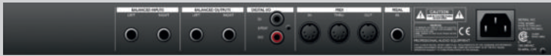
Balanced Jack Analog Inputs Balanced Jack Analog Outputs Digital S/PDIF Input/Output MIDI In, Thru, Out External Control Input Power Input 100 - 240V
