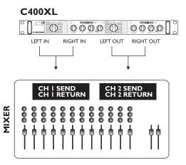
In this example the C400XL is used in Dual Mono mode as two 100% independent mono engines on two separate channels. The two engines have no influence on each other.
