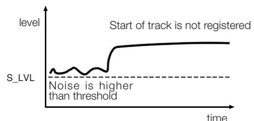
Synchronized recording stops when the sound level drops below the threshold for five seconds:
