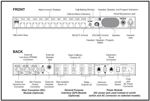
FIGURE 3. KP-12 Keypanel Reference View (Push-button version shown).
