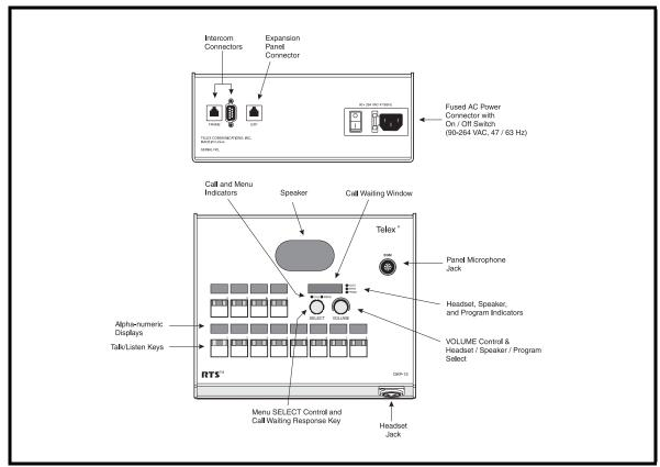
FIGURE 2. DKP-12 Keypanel Reference View (Push-button version shown).
