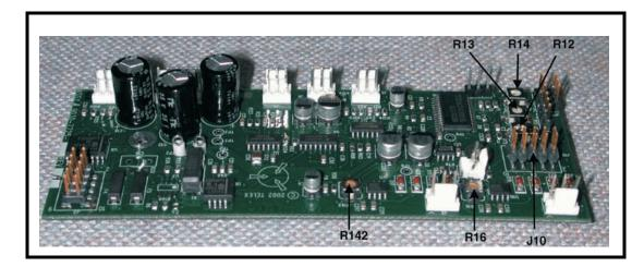
The new audio transmit board (9030-7725-500), if used with the new controller board (9030-7725-000) has digital control for compression setting and Mic gain setting through the master volume encoder of the KP-12.
