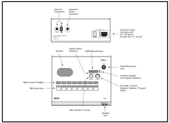
FIGURE 1. DKP-8 Keypanel Reference View (Push-button version shown)
