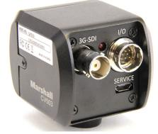
**CV-PT-HEAD** comes with a patch cable for Marshall cameras. The table below is used if a Male connector is fitted on the camera. ie. if the connector on the camera itself has pins – like in the picture.
