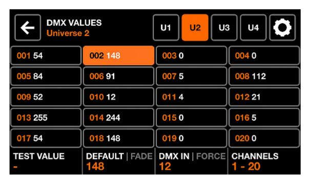
The DMX Values screen displays the current value of each DMX channel. It allows for the value to be changed for testing purposes, and for channel settings to be adjusted.
