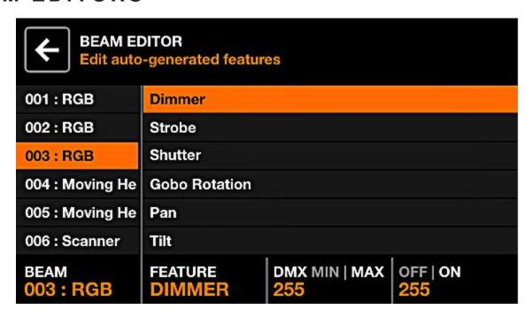
Advanced: each fixture is split up into beams and beam features. Each beam feature contains min/max and on/off values which are set automatically by Wolfmix. These values are calculated by the fixture profile and should not require changing. However if there is a fault with the fixture profile or a special case, some of these values can be edited via the Beam Editor screen.
