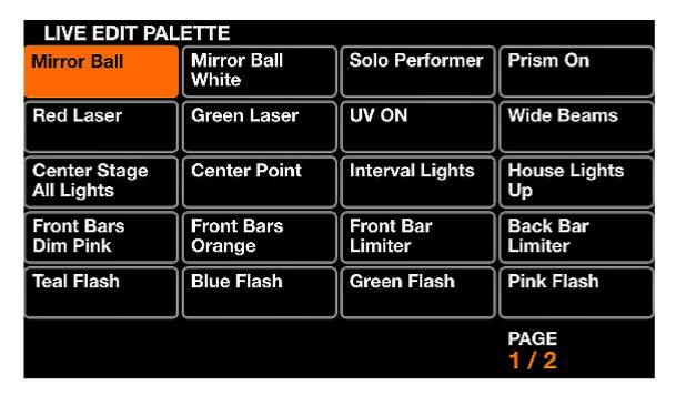
The Live Edit screen contains a palette of twenty buttons which can be used to recall a value on any channel. These values override all effects and other static values. Live Edits are layered in order, therefore if two live edits have values on the same channel, the buttons towards the bottom will take priority.
