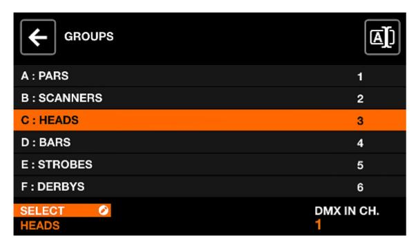
Each fixture is linked with a group. Effects, sub-dimmers, static colors and positions are applied to each group. Wolfmix supports up to 8 groups. 4 can be displayed at a time with groups A-D and E-H toggles by shift + hitting the BPM TAP button. Each group can be assigned a name and a DMX input channel on the Groups screen.
