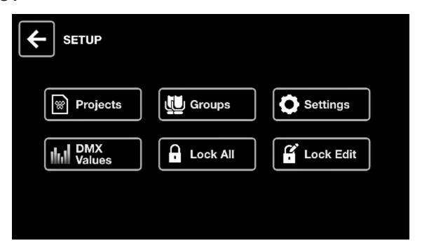
The Setup screen is accessed by tapping the icon to the top right of the Home screen to the left of the Fixture icon.
