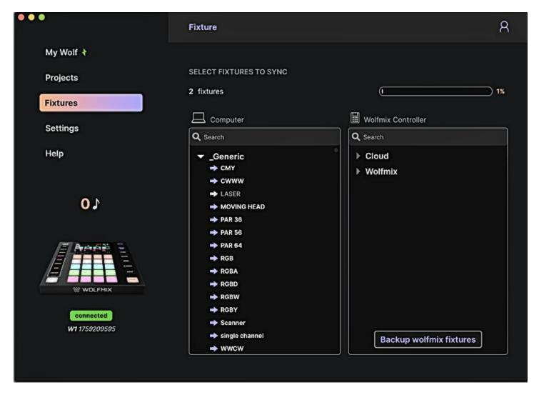
Fixtures on the computer and in the cloud are displayed on the left and fixtures in the Wolfmix controller are displayed on the right.
