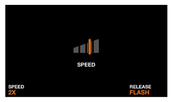
The Speed flash effect multiplies the speed of all effects by the set multiplier. The effect is released according to the set release mode.
