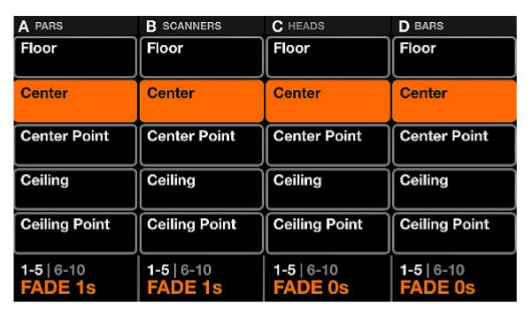
The static position screen contains a palette of five positions per group. Selecting a position will override any playing move effects on the group and set all fixtures in the group to the selected position.
