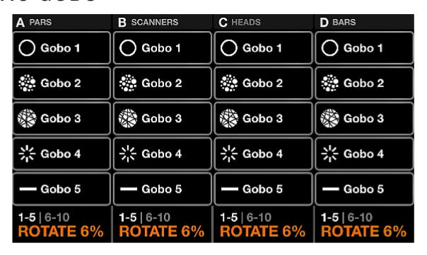
The static gobo screen contains a palette of 10 gobos per group. Selecting a gobo will recall the gobo on all fixtures in the group. If a gobo is not selected, the open gobo will be triggered. When a fixture is added to a project, the Wolfmix will try to group similar gobos together within the first 5 palette items.
