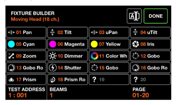
The fixture builder is used to create fixture profiles. A fixture profile is a list of channels and features associated with a particular fixture.
