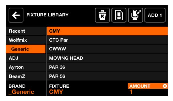
The fixture selection screen shows all available fixture profiles on the controller, ordered alphabetically by brand and fixture.
