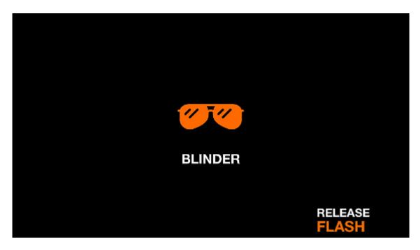
The Blinder flash effect sets all dimmers to 100% and all color mixing channels to white. The effect is released according to the set release mode.
