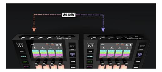
Finally, be sure both Wolfmix's have the same Project loaded, then head over to the Settings screen, scroll to WLINK input mode, and select WOLFMIX.
