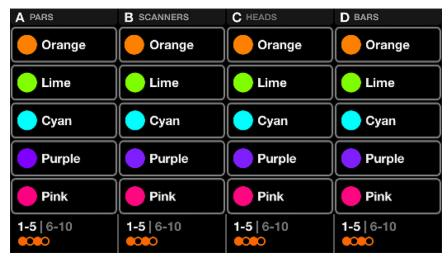
To change default colors, shift + hit one of the color buttons, select a new color and then hit the flashing button to save the changes. (Top tip: Tap the RGBWAU button to the top right to have independent control over your Amber and UV channels.)
