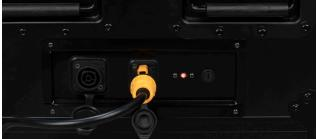
. AC Power In/Out built-in - Daisy chain power
