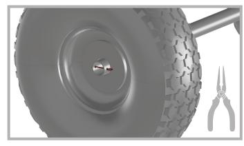
Finish with inserting cotter pin into hole and bending ends backward at 90 degrees with pliers.
