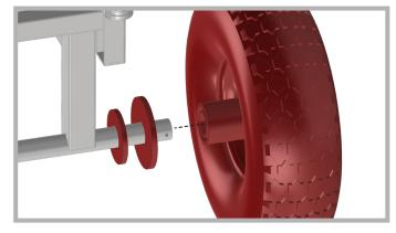
Gently slide small washer, then large washer onto rear axle. Then slide wheel onto the axle.
