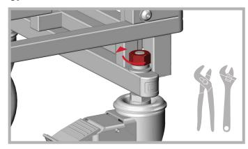
Finish by tightening nut onto caster using wrench and channel lock pliers. Tighten firmly until lock washer no longer rotates.
