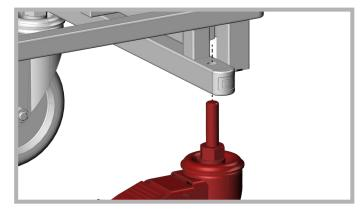
Slide top of swivel caster upwards into the front axle hole.
