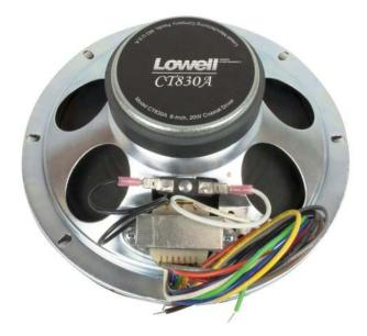
shall be zinc-plated to resist rust and corrosion. The speaker shall have a mounted transformer with primary taps at .25, .5, 1, 2, 5W @70/25V. The assembly shall be capable of producing a uniform audible frequency response over the range 57Hz-13.5kHz ( $\pm$ 6dB); 44Hz-20kHz ( $\pm$ 8.4dB) with dispersion angle of 80 degrees @2000Hz (-6dB). Average sensitivity shall measure 97.4dB (SPL at 1W/1M). Assembly mounting depth shall not exceed 3.2".
