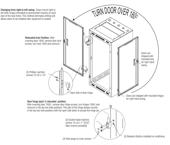
Door hinge pin (part 2) mounts to cabinet without drilling. The second part of the door hinge (pin) is always field installed to factory mounted nutserts. Nutserts are located on the front left and right of cabinet.
