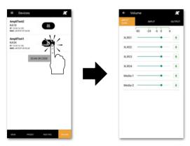
3. Input and output levels adjustments are always available: input gain adjustments are available only in 4-channel units. The media player level can always be adjusted via the built-in web app.
