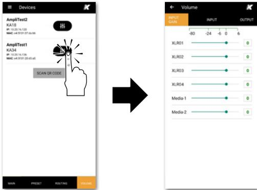
3. Input and output levels adjustments are always available: input gain adjustments are available only in 4-channel units. The media player level can always be adjusted via the built-in web app.
