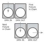
2. Connect the end of the cable coming from the first fixture which will have a female connector to the input connector of the next fixture consisting of a male connector. Then, proceed to connect from the output as stated above to the input of the following fixture and so on.
