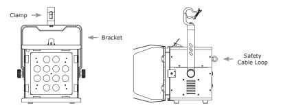
Mount the fixture using a suitable "C" or "O" type clamp. The clamp should be rated to hold at least 10x the fixture's weight to ensure structural stability. Do not mount to surfaces of unknown strength, and ensure properly rated rigging is used when mounting fixtures overhead.
