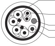
Conductor:2P\*30AWG(7/0.10 Tinned Copper) Isulation: 90.79 (LDPE) Shield: Alumimium Foil+Mylar P1: White & BLUE P2: White & BLUE Drain: (7/0.10±0.008mm Tinned Copper)
