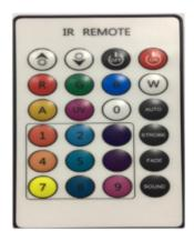
**UP/DOWN ARROW:** Scrolls through Auto Modes and Sound Modes, or adjusts intensity for Red, Green, Blue, White, or UV lighting display modes.
