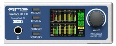
When the Global Level Meter screen is shown, the rotary encoder sets the monitoring volume of Main Out directly at the device. Pushing the button will change to Phones volume control, as indicated in the right lower corner of the screen.
