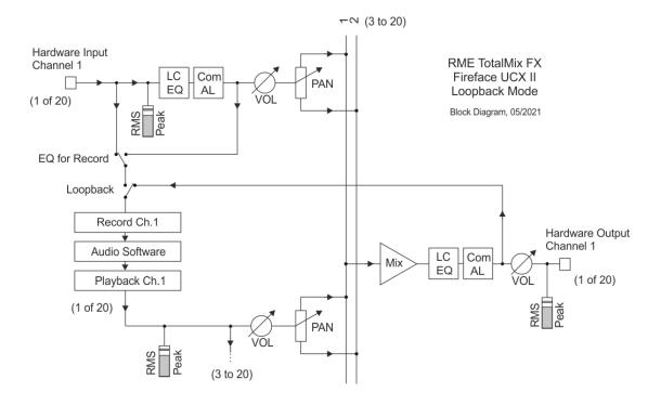
As each of the 10 stereo hardware outputs can be routed to the record software, and none of these hardware inputs get lost, TotalMix offers an overall flexibility and performance not rivalled by any other solution.
