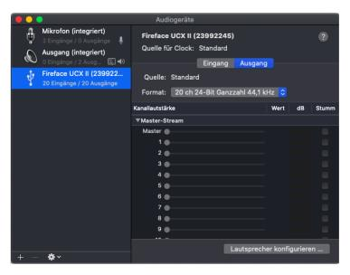
With 8 and 14 channels chosen up to 192 kHz sample rate can be used. Under iOS 192 kHz is not possible, as there exists no way to select the second or further *Alternate Setting* on the record side. iOS and all apps always use the first setting, 20 channels, which limits the sample rate for record and playback to 96 kHz.
