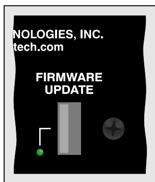
Figure 18. Detail of Model 792 back panel showing the USB receptacle
