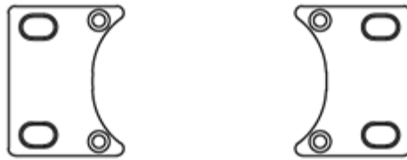
Rack ear accessories for installing the PWPP RM P8 unit into a 19" equipment rack.
