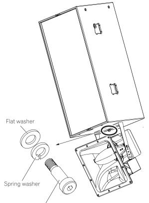
Using the dedicated screws, washer, and spring washer included with the XY-2, firmly attach it to the bottom threaded point of the XY-3B. - the flat washer should be in contact with the yoke. Tighten the bolts to ensure a solid fit. Once the desired angle of the loudspeaker is set, tighten the bolts on the yoke to lock the position in place.
