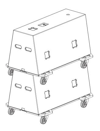
Attach the wheel board to the front of the enclosure using the butterfly latches on both sides of the wheel board.
