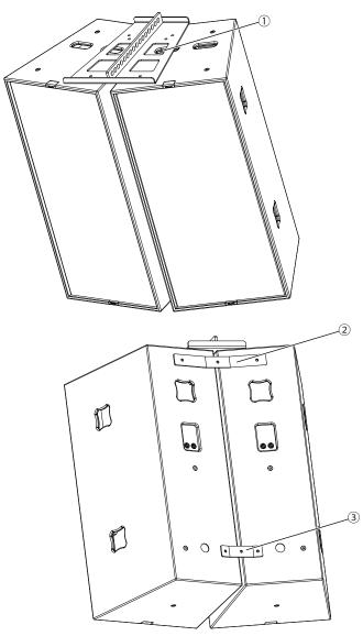
Using the supplied M10 socket head bolts, bolt through the CP-XY3DF1 the top-plate and two rear-plate into the enclosures. Ensure that both the flat and spring washers are used - the flat washer should be in contact with the top-plate. When assembling cluster of two XY-3s using the CP-XY3DF1, XY-2s can be attached to the bottom of enclosures.
