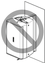
The outer yoke of the cradle is not horizontal to the wall
