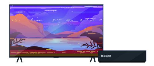
Check the antenna and input cable connections.
