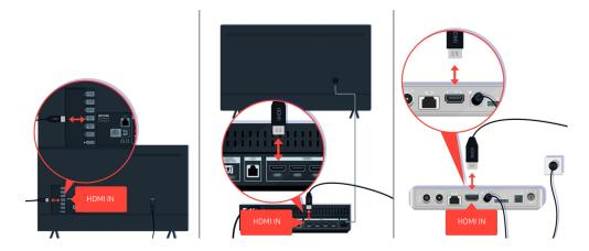
Check the antenna and HDMI cable connections.
