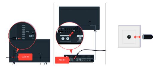
Check the antenna and input cable connections.
