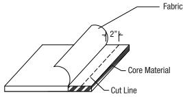
Clamp a straight edge at the cut line. Cut through the core, following the straight edge.
