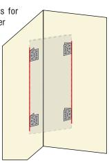
For vertical corners align the panel ¾" above its target height and press down at a 45° angle until flush with the wall. For horizontal installations apply Tubetak Pro adhesive to the impaling clip face, not to the points.
