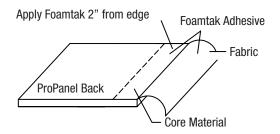
At the corners, trim the back and edges with sharp scissors. Leave enough fabric to close each corner. Install the ProPanel.
