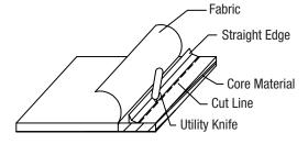
Cut the fabric, leaving two inches more fabric than the core and edge thickness.
