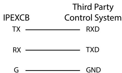
The RS232 control ports require a standard straight-through serial cable for operation. The default settings for the RS232 ports are:
