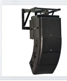
The Steerables Line Array Wall Mount installs and aims line arrays on either side of a stage or building. It's heavy black powder-coated steel framework assures safe installations and installs permanently. Line Arrays suspend from their own overhead rigging points, which allows for the desired tilt angle. Pan angles, up to 45 degrees left or right are achieved by way of an upper cross arm to aim the line array into the desired angle. An outdoor version, the SAS-500-WM-G, comes
